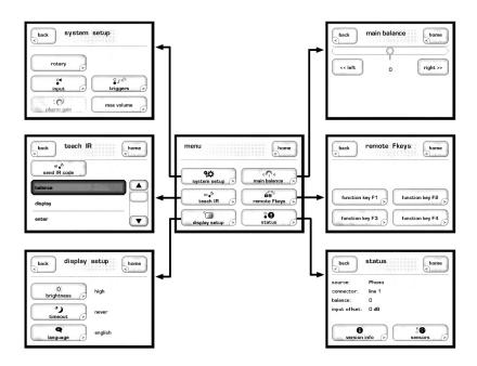
Pressing the front panel **Menu** button to the left of the **LCD touchscreen** brings up a comprehensive *main menu system*, the top two levels of which are shown above. This menu provides access to many installation-specific features that let you customize how the CP-500 works within the context of your particular system.
